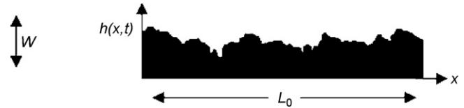
Fig. 6. A schematic sketch of the definition of the statistical width W of a contact line, as the second moment of the front position h(x,t) , for a given time.
