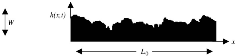
Fig. 2. The function h(x,t) for describing the interface characteristics, representing a top view of the experiment. The width W satisfies Eqs. (1) and (2).
